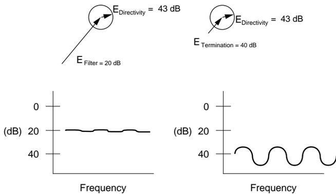
**Figure 1: Vector Signal Addition**
